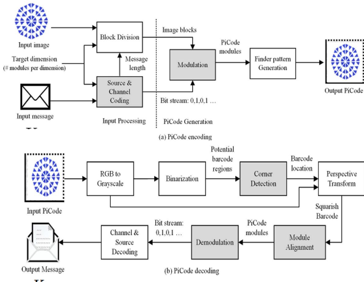
Fig. 2. Block diagram of picode encoding and decoding
