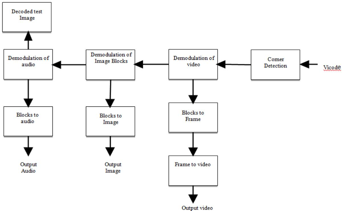
Fig.5.Decoding processes of Vicode
