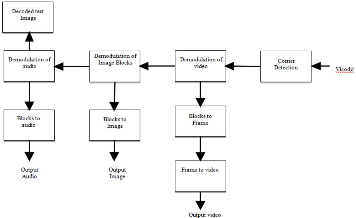
Fig.5.Decoding processes of Vicode
