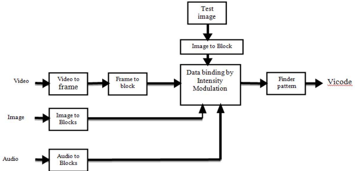
Fig.4.Block diagram of vicode generation.
