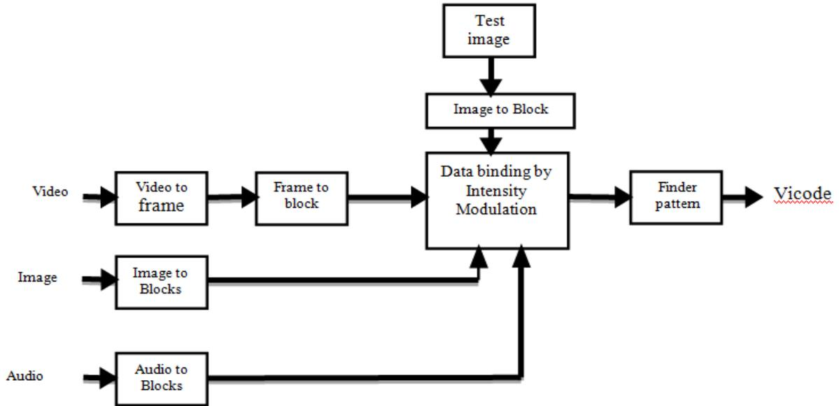
Fig.4.Block diagram of vicode generation.
